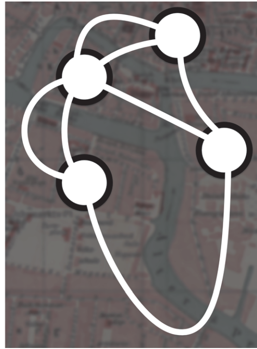
FIGURE 1-1: In the seven bridges of Königsberg problem, Leonhard Euler explored whether each bridge could be crossed only once. On the left is a map showing the seven bridges, and on the right is the graph equivalent.
